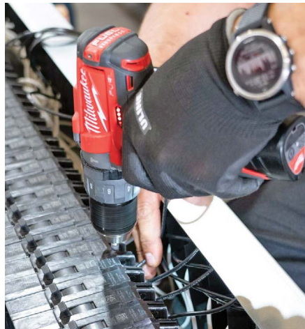
AEAMC staff builds specialized distribution panels for computer servers used in cryptocurrency mining.
